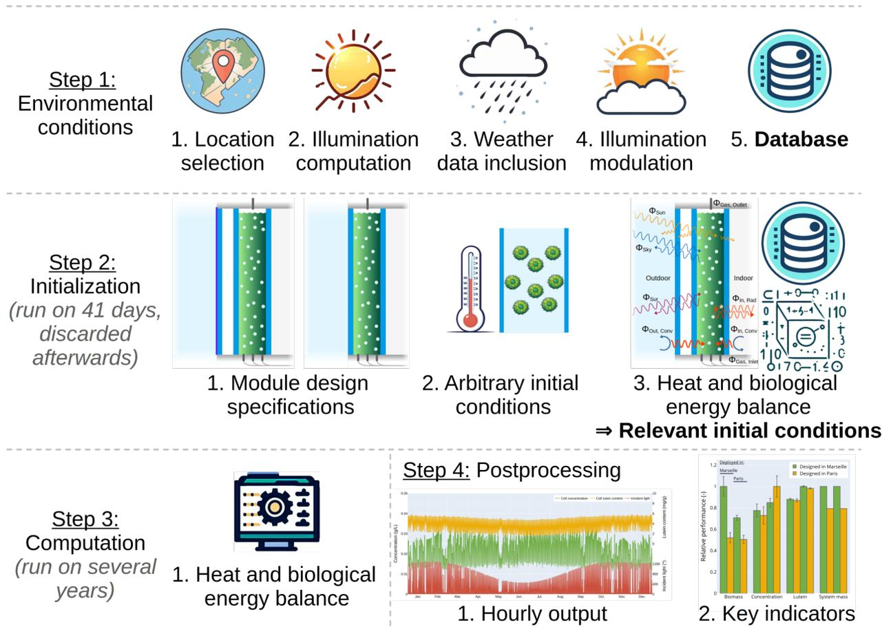
Fig. 2. Numerical workflow
