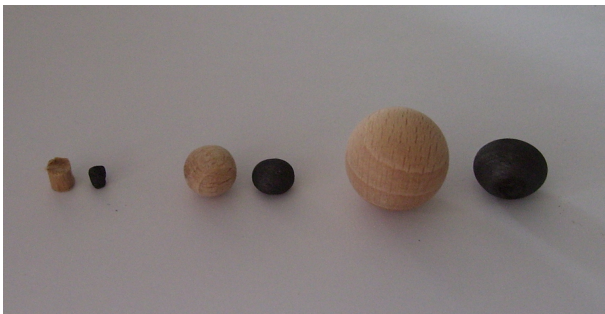
Fig. 4. Samples before and after exposure. From left to right: 5 mm cylinder, 10 mm sphere and 20 mm sphere
