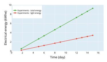
**Figure 4.** Total process consumed electrical energy and light consumed electrical energy over time. Measurements started after 24 h. Fitted values: total energy (kWhe) =  $0.662 \times \text{time}$  (day)  $\pm 0.000$ .  $R^2 = 1$ . Lighting energy (kWhe) =  $0.244 \times \text{time}$  (day)  $\pm 0.000$ .  $R^2 = 1$ .
