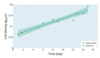
**Figure 2.** Biomass density over the first part of the run (from 50 mL samples) and its linear fit. Culture medium volume: 52 L. Fitted values: density  $(g_{DW}/L) = 7.81 \times 10^{-3} \times \text{time (day)} \pm 57.8 \times 10^{-3}$ .  $R^2 = 0.914$ .
